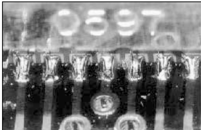
Figure 7.12 x-axis Misalignment Self-corrected after Reflow.
